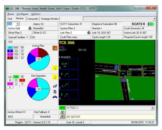
Figure 3: SCATS graphic of Thomas St/Meath St junction with four phases
